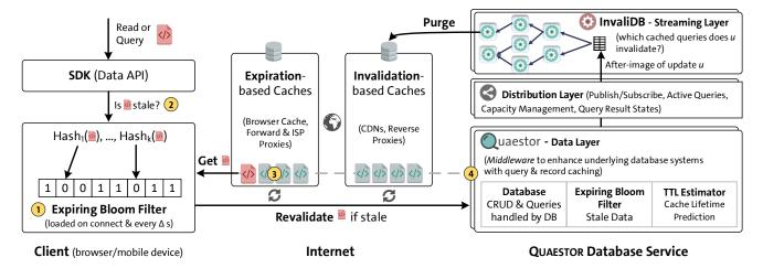
Figure 3: QUAESTOR: client-server architecture and components.
